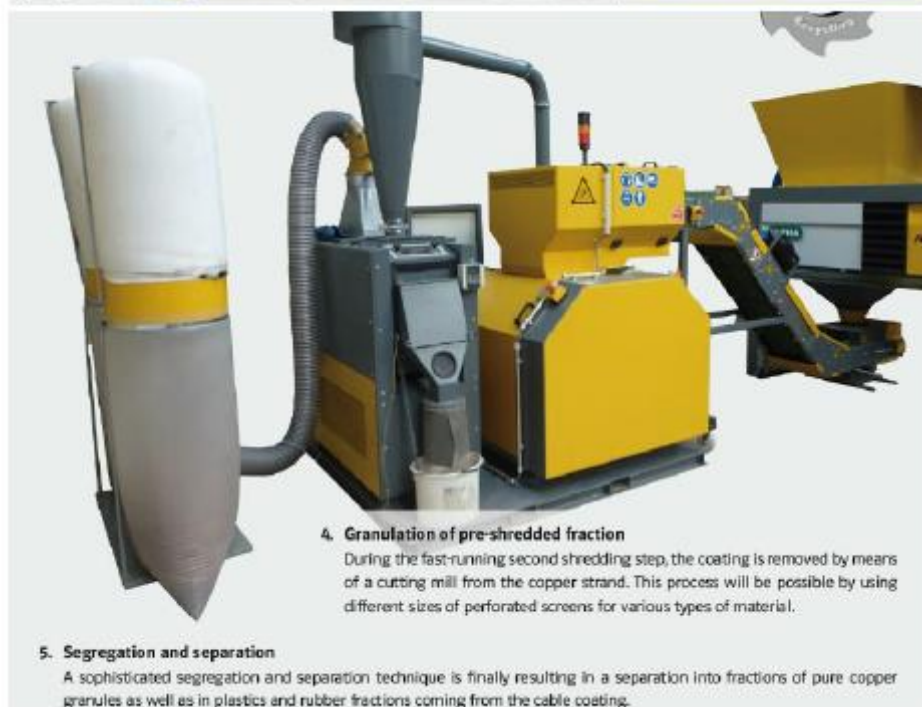
Figure 3-14: Detailed process flow of cable waste shredding 14 .
